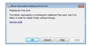
The Rotational Free End block has no parameters.
